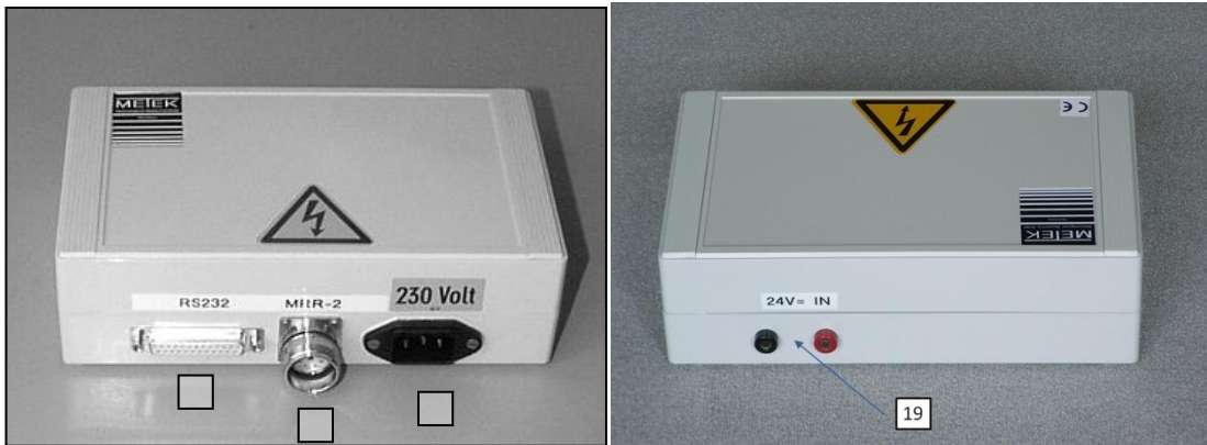
Figure 4: Junction Box Left:Front Side, Right: Back Side
